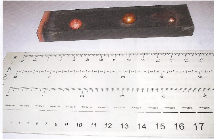
Figure 2: Wettability problem of copper on graphite boat
