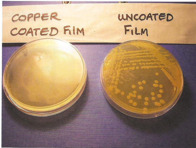
Figure 7: Effect of copper metallized and non-metallized PET film on bacterial growth
