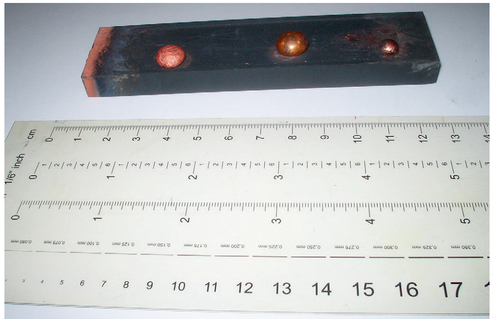
Figure 2: Wettability problem of copper on graphite boat
