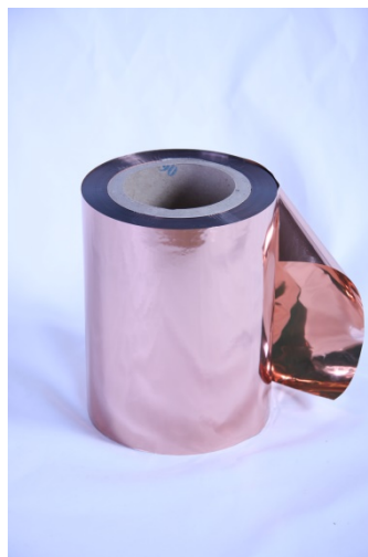
Figure 9. Copper metallization inside a standard web metallizer
