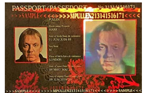
Example of full colour photopolymer reflection holographic passport overlay film with individual holographic data authentication.
